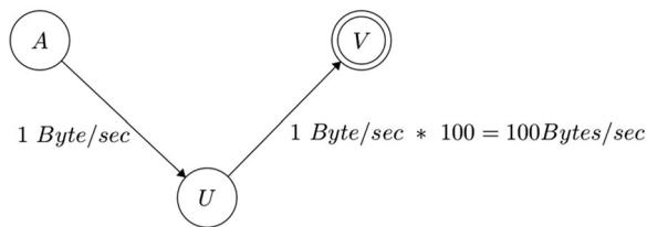
**Figure 1.** Illustration of a reflective DDoS attack where the attacker A uses a UDP amplifier with an amplification factor of 100 as a reflector. The attacker sends a message to U, with a spoofed IP address that makes it look like it was the victim V that sent the message, resulting in the victim V getting the amplified response from U.
